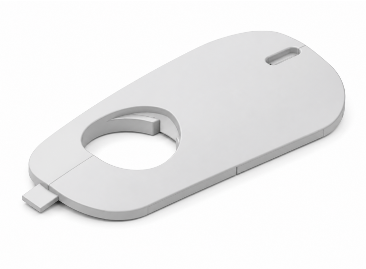
Figure 7: The custom GNSS/Magnetometer enclosure, designed to physically isolate the compass from internal electromagnetic interference.
