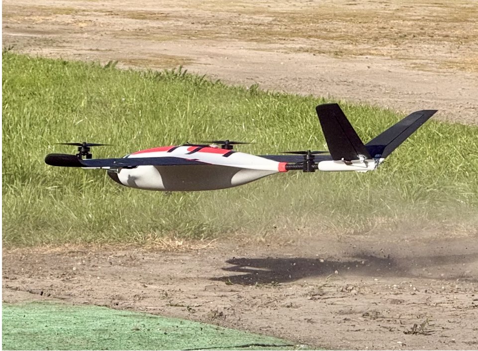
Figure 25: Balrog v1 during early hover testing. The prototype successfully demonstrated VTOL operation and completed its first transition into fixed-wing flight.
